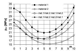
Figure 4 Critical load distribution versus buckling mode for plates with homogeneous and heterogeneous one-layer facings
