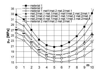
Figure 5 Critical load distribution versus buckling mode for plates with homogeneous and heterogeneous one-layer and two sublayers facings
