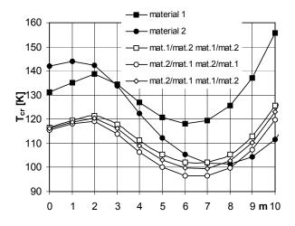
Figure 9 Critical temperature distribution versus buckling mode for plates (SC-SC) with homogeneous and heterogeneous one-layer facings, thermally loaded on inner edge
