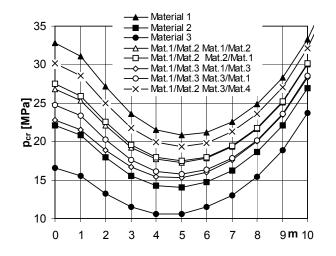
Figure 6 Critical load distribution versus buckling mode for plates with homogeneous and heterogeneous ten sublayers core
