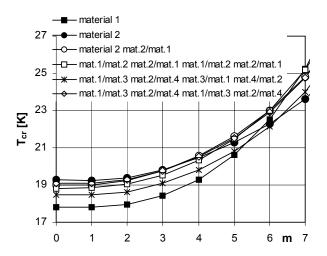
**Figure 11** Critical temperature distribution versus buckling mode for plates (C-C) with homogeneous and heterogeneous two-layers facings, thermally loaded on inner edge
