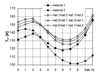
Figure 10 Critical temperature distribution versus buckling mode for plates (SC-SC) with homogeneous and heterogeneous one-layer facings, thermally loaded on outer edge
