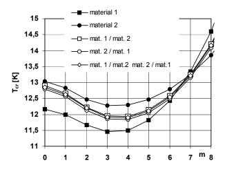
Figure 7 Critical temperature distribution versus buckling mode for plates (C-C) with homogeneous and heterogeneous one-layer facings, thermally loaded on outer edge
