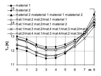
Figure 8 Critical temperature distribution versus buckling mode for plates (C-C) with homogeneous and heterogeneous two-layers facings, thermally loaded on outer edge  $\,$
